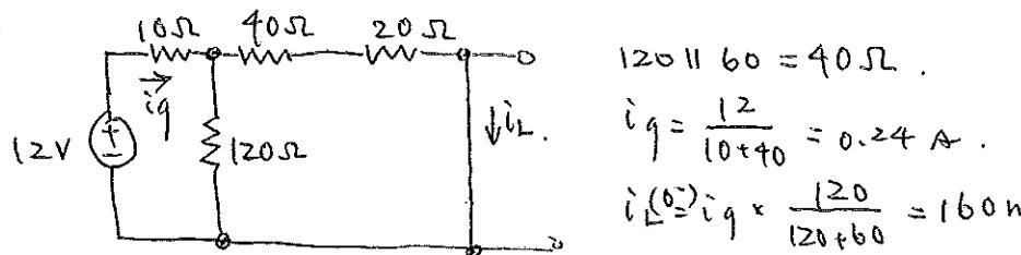
$t=0^+$ ,  $i_L(0^+) = 160 \text{ mA}$ . (Current cannot change instantaneously).
