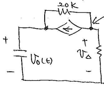
$$\text{KCL: } \frac{V_a}{5000} + \frac{V_a - V_o}{20000} + 2.5 \times 10^{-4} V_o = 0$$
