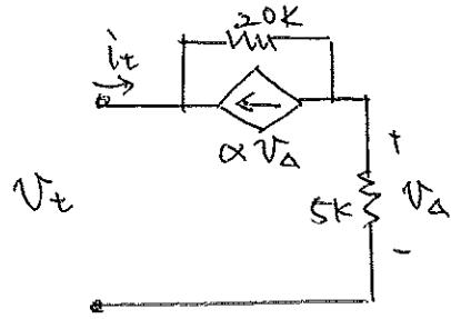
APPLY test voltage  $V_t$  to solve for  $R_{th}$ ...
